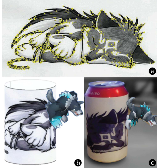
Figure 2: The pairing between the digital and the physical uses Vuforia. a) Yellow crosses are the unique features for MR pairing. b) The image can be wrapped in a cylindrical shape. c) A can that is detected with the digital wolf attached to it. The image was created and licensed by Deviant Art 1 .
